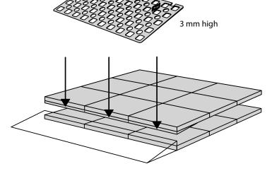
When you connect a platform and a ramp, remove the Ramp Adjuster from the ramp, and use it to adjust the platform as shown here:
