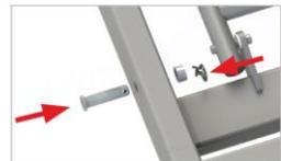
Clevis pin, spacer, and R clip fitting
